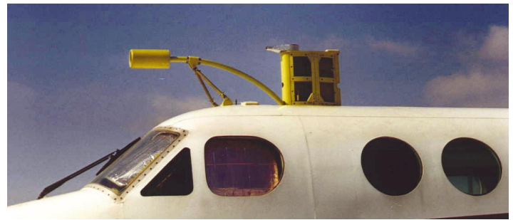
Dust collector mounted atop research aircraft.
